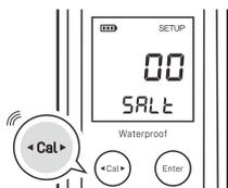
2. Press the **Enter** key until the display shows °C/CAL or °F/CAL.
