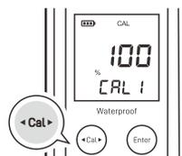
1.2 Hold the dissolved oxygen electrode in the air at 100% relative humidity or place the electrode into the air-saturated water for about 10 minutes. Press the **Enter** key to begin the calibration.
