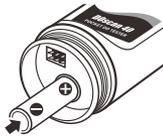
3. Push the connector into the tester and twist the connector collar clockwise until tight.
