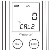
2.2 Place the dissolved oxygen electrode into the zero oxygen solution for about 10 minutes, press the **Enter** key to begin the calibration. When the reading has stabilized, the tester will show *End*. Calibration is completed.
